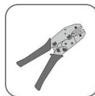
Terminal crimping tool (10 mm 2 , cold-pressed terminal)
